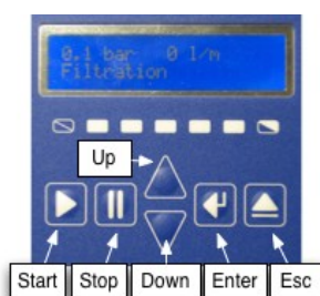
Picture 13: Control Panel of the Sec-cua UF unit
